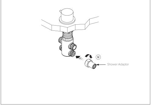
10. Once the diverter is fully installed, the shower adaptor (U) can be screwed onto it's required outlet port.
