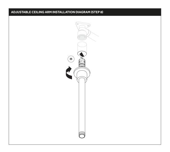
8. Apply a suitable sealant or sealing tape to the threaded tail. Screw the threaded tail into the female wall outlet (H).
