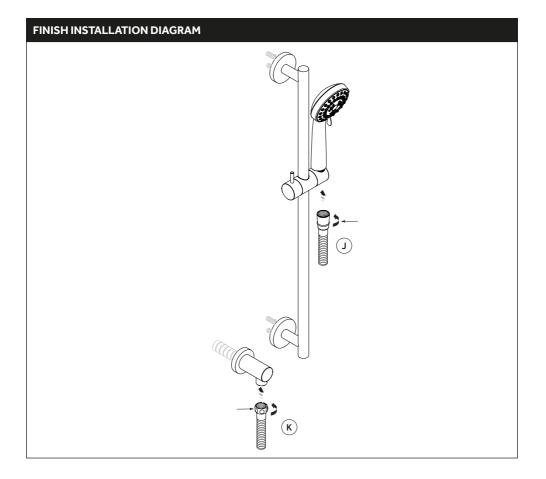
Use the provided shower hose to connect the handshower to the wall outlet bracket and slide rail handshower. The conical end of the hose should be screwed onto the threaded end of the handshower (J). Screw the hexagonal end of the shower hose onto the outlet port on the underside of the shower bracket (K).
