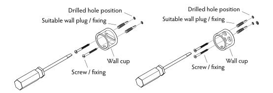
10. Offer the towel warmer to the wall cups, passing the cable through the drilled hole. Locate the towel warmer and tighten the grub screws using a 3mm hexagonal key.
