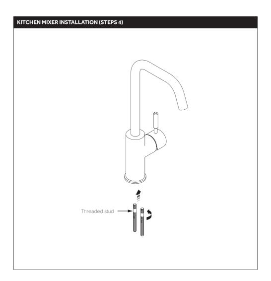
4. Screw the threaded studs into the threaded holes in the underside of the mixer.
