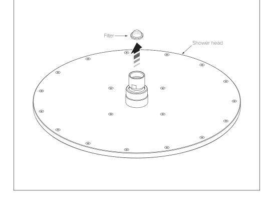
1. There is a filter fitted in the inlet of the shower head. If water flow from the shower head has reduced, it may be an indication that the filter requires cleaning.
