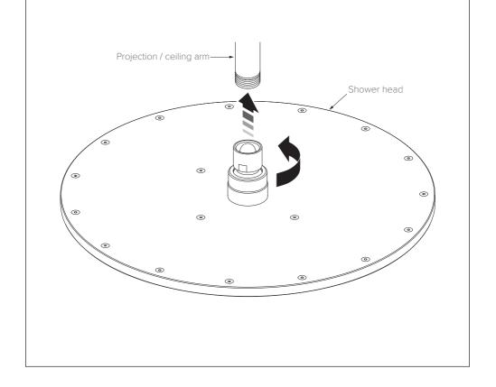
2. Before screwing the shower head onto the shower arm ensure that the pipework has been flushed of debris and that there are no leaks.
