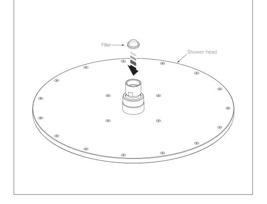
1. After removing the shower head from its packaging, ensure that the filter is inserted into the swivel inlet on top of the shower head. The dome of the filter should face upward.
