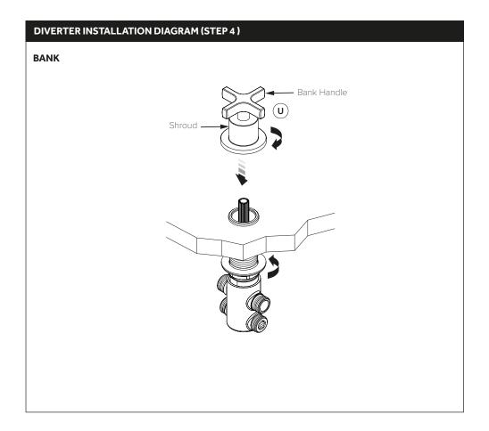
4. For Bank diverter trim asembly, locate the Bank handle (U) onto the spline and secure by screwing the shroud onto the diverter body
