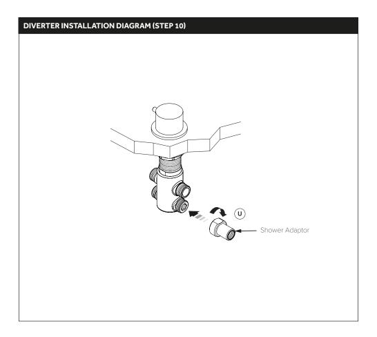
10. Once the diverter is fully installed, the shower adaptor (U) can be screwed onto its required outlet port. Please refer to 'Making the Connections' sections for port details.
