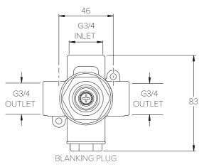
The diverter is supplied with a blanking plug fitted. This can be removed if an additional supply inlet is required.
