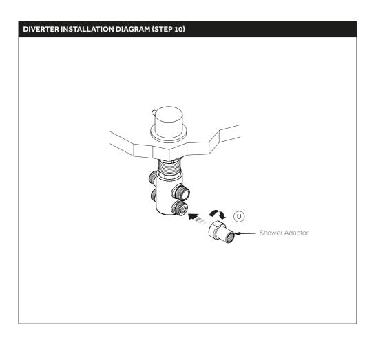
10. Once the diverter is fully installed, the shower adaptor (U) can be screwed onto it's required outlet port.
