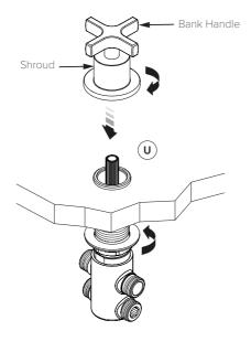
4. For Bank diverter trim assembly, locate the Bank handle (U) onto the spline and secure by screwing the shroud onto the diverter body
