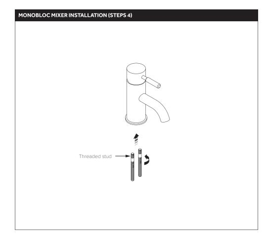
4. Screw the threaded studs into the threaded holes in the underside of the monobloc mixer.
