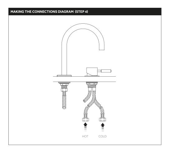
4. Check all connections for leaks before concealing pipework and finishing installation.
