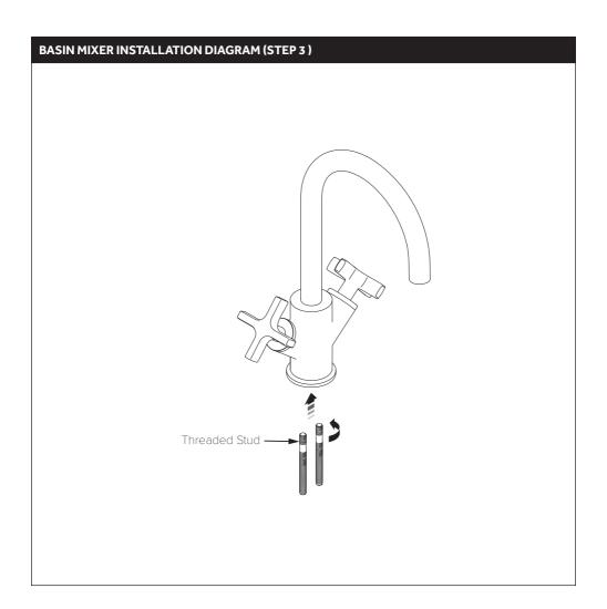
3. Screw the threaded studs into the threaded holes in the underside of the basin mixer.
